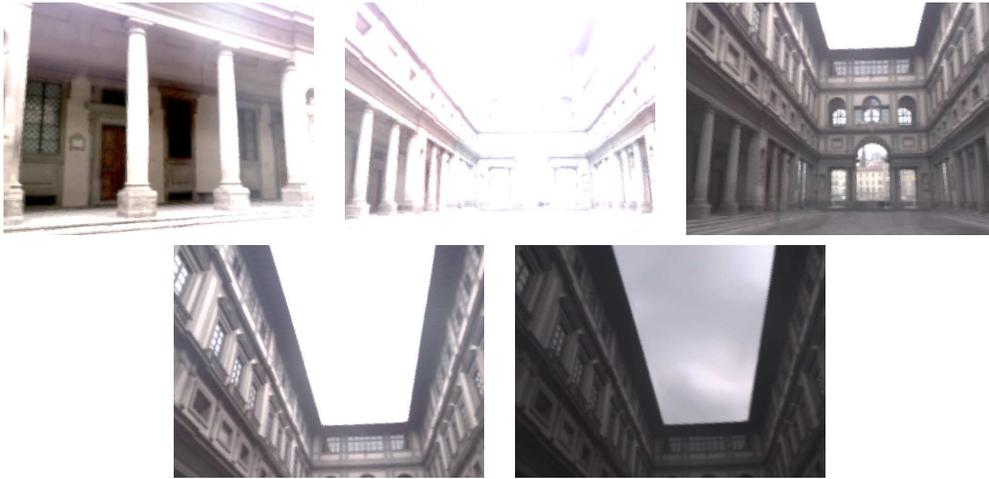
**Fig. 2.** Screen snapshots from our high-dynamic range panorama viewer. The viewer implements our HDRTM technique allowing these results to be rendered interactively at 50 Hertz at  $640 \times 480$  pixels with 4x antialiasing. The exposure changes by a factor of 100 over these 5 images.
