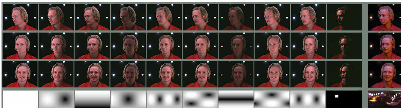
Fig. 1: An actor stands within a sphere of inward-pointing LED lights as elements of the spherical harmonic lighting basis (bottom) are projected in rapid succession during each extended frame. Linear combinations of the frames produce novel illumination on the performance according to a sampled lighting environment (right).
