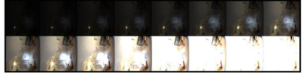
**Figure 5: An ILF high-dynamic range image series,** is a sequence of 16 images with increasing exposure time from left to right. The image series is used to reconstruct the high-dynamic range measurement of incident illumination for a specific location in the capturing plane.
