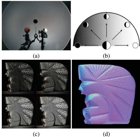
**Figure 9:** *Acquiring normals for a highly specular surface. (a) Reflective hemisphere to create continuous gradient illumination, showing the viewing aperture, subject, and half-covered light bulb. (b) Diagram of a half-covered light bulb producing gradient illumination. (c) Left, top, front, and full gradient illumination conditions on a polished obsidian sculpture. (d) Computed normal map from the specular reflection.*
